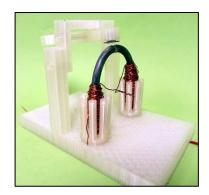
With appropriate scaffolding, middle school students are capable of designing a working reciprocating motor based on the same principles as the original "electromotive device" developed by Joseph Henry. This affords opportunities for novices to design an initial solution to the challenge, with ample scope for refinement.
