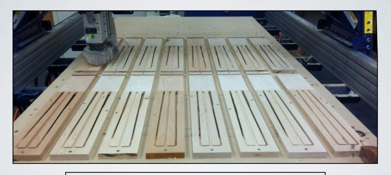
16 GUITAR NECKS BEING CUT ON A SHOPBOT CNC MILL
